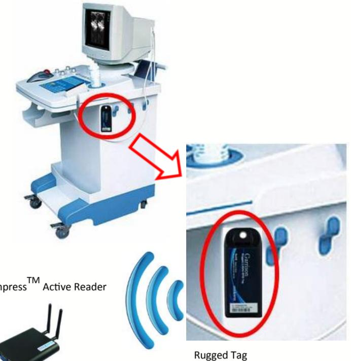
**2** Tag ID of each equipment would be sent to the reader periodically for real time tracking.
