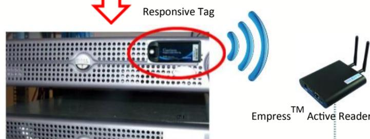
**2** Tag ID would be sent to the reader periodically to keep track of the servers. The tamperproof sensor status of each tag on each server is instantly sent to the system.
